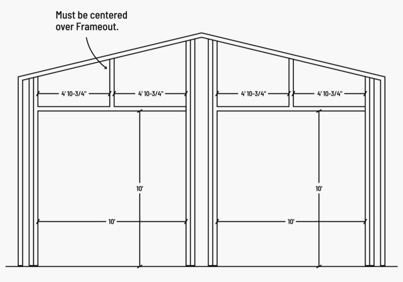
Frameouts for overhead door example Make Frameout 1 inch less wide than actual door.
